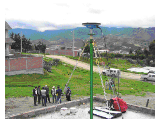
Fig. 4. Differential GPS monitoring station.
